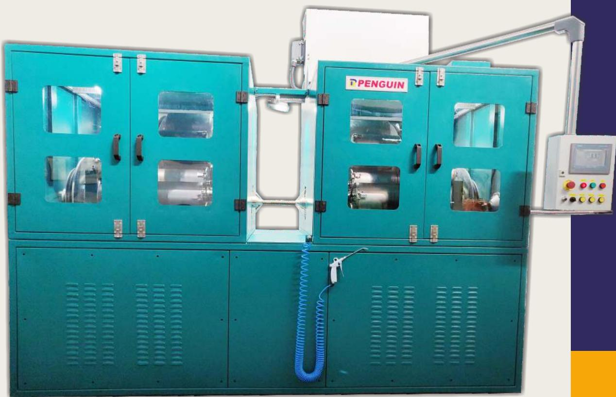
**P**ENGUIN Spiraling machine is used in the construction of spiral structure of yarn over rubber hose. Spiraling is done to increase the strength of rubber hose. The spiraled rubber hose can be used in production of low and medium pressure hoses.
