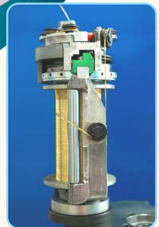
Wire carriers with Preformer
