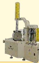
MINI ROLL WRAPPER Productivity: 30-75 rolls/hour Applications: Retread rubber rolls, tyres, coils, mini paper rolls, flexible packaging rolls, spools...
