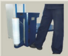
Leg crush sensor for operator safety
