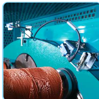
Bobbin empty and Wire cut sensors
