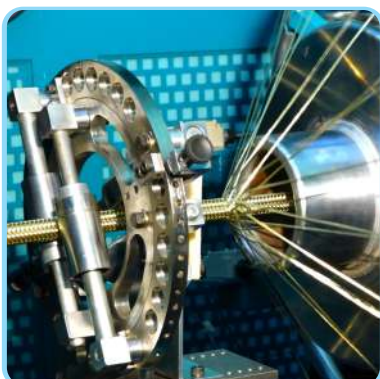
Adjustable guide rollers for different hose diameters
